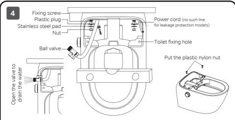
After the toilet is close to the wall, use a gradienter to measure the product to keep the product in a horizontal position. Then put a plastic plug and a stainless steel gasket on the fixed screw in turn, and then tighten the nut. Then connect the ball valve to the head of the outlet pipe and pass water to clear waste. Then put plastic nylon nut in the toilet fixing hole.
