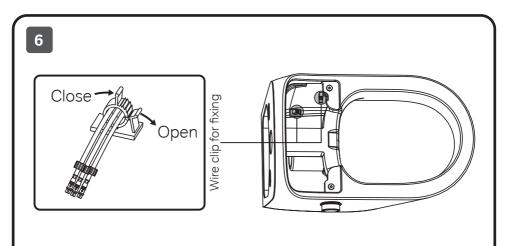
After the ambient light wire, knob wire and microwave induction wire are connected, arrange the wires and put them into the wire clip, and then press and hold the wire clip in the direction of closing indicated by the arrow. When you need to take out thewire, press the wire clip in the direction of opening indicated by the arrow.
