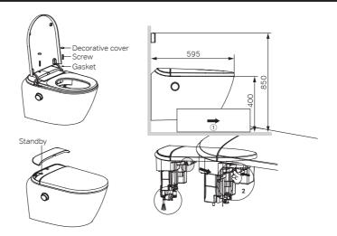
Fix the electronic seat on the top of ceramic, tighten it with the fixing screw, and install the decorative cover. after installation, take out the package in the direction of the arrow  ${\bf 1}$  in the figure. The remote control is installed at a distance of about 850mm from the ground, which is easy for users to remove it. When not in the use for a long time, press in the direction of arrow  ${\bf 2}$  to drain the residual water in the pipe.
